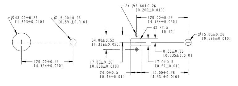
Recommended Glass Mounting Hole Pattern Recommended Steel Mounting Hole Pattern
